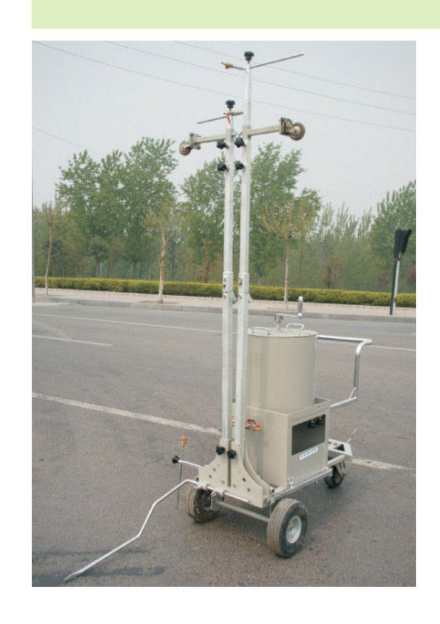
If pre-marking by vehicle before the road marking, the cost of the vehicle input is usually high. Also, the marking work is often affected because of the pre-marker's not timely in place. DAYU brand hand- push pre-marker can mark the pre-marking freely according to the requirements of construction and can accomplish 1~4 lines independently, which greatly improves the construction efficiency.
